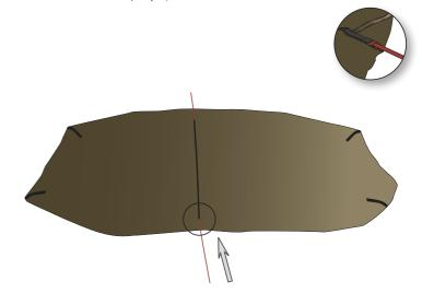
Fix the pole ends into the webbing eyelets. Secure the tent to the ground by attaching pegs onto each guy rope ring, starting in the end and facing the wind. Pull the guy rope rings in the opposite end towards you. Erect the tent and secure with pegs.
